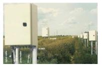
Field installation of TDR data logger
